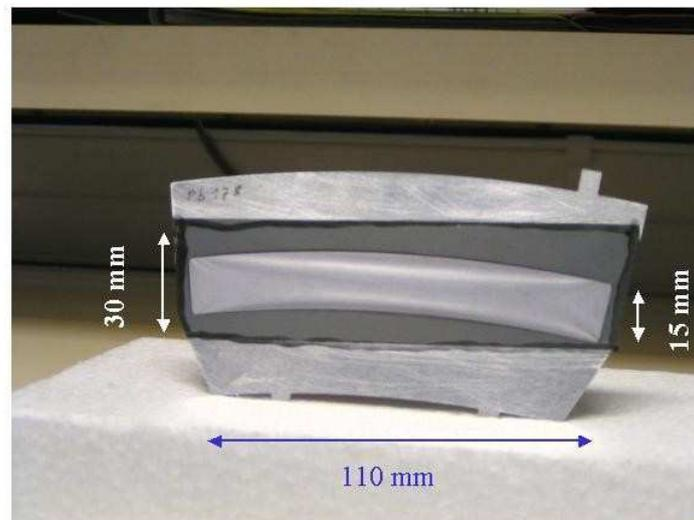
Figure 3: Enriched  $^{208}\text{Pb}$  target, 15 mm in height, 100 mm long: C  $35 \mu\text{g}/\text{cm}^2$  + Pb  $350 \mu\text{g}/\text{cm}^2$  + C  $5 \mu\text{g}/\text{cm}^2$ .
