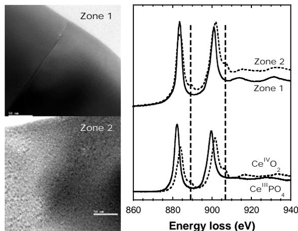
**Figure 7.** TEM observation and cerium EELS spectra of  $\text{M}_{4,5}$ -edge fine structure of  $\text{CeO}_2$ - $\text{CaO}$ - $2\text{NH}_4\text{H}_2\text{PO}_4$  mixture fired at  $1400^\circ\text{C}$ .
