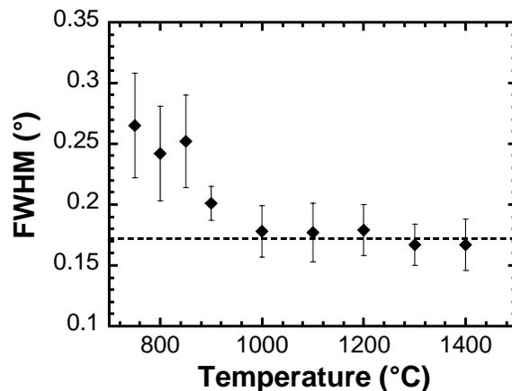
**Figure 3.** Average FWHM of the main XRD lines (i.e.  $\bar{1}11$ ,  $20\bar{1}$ ,  $120$ ,  $012$ ,  $20\bar{2}$  and  $112$ ) of  $\text{Ca}_{0.5}\text{Th}_{0.5}\text{PO}_4$ , versus synthesis temperature.
