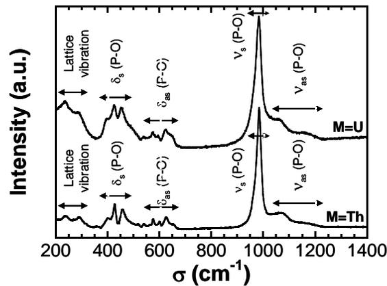
**Figure 2.**  $\mu$ -Raman spectra of  $\text{Ca}_{0.5}\text{M}_{0.5}\text{PO}_4$ .
