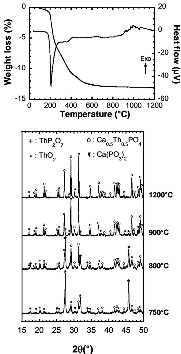
**Figure 1.** Thermal analysis under argon and X-ray diffraction analysis of a ThO<sub>2</sub>-Ca(HPO<sub>4</sub>)·2H<sub>2</sub>O-NH<sub>4</sub>H<sub>2</sub>PO<sub>4</sub> mixture.
