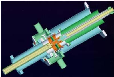
Figure 4: Sketch of the 704 MHz high power coupler.
