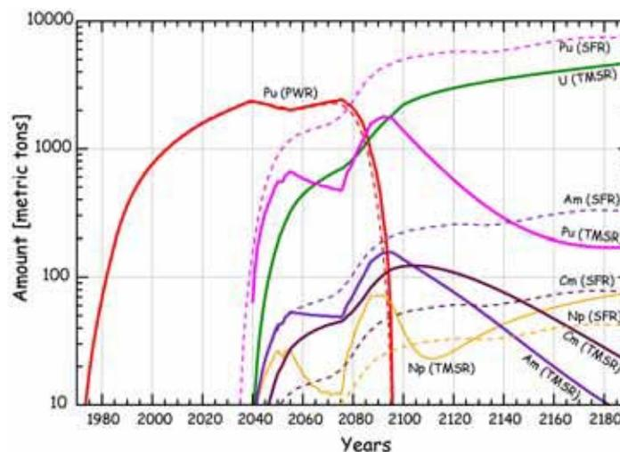
Fig. 5: Stockpiles of transuranic elements and  $^{233}\text{U}$  for two deployment scenarios: combination of LWRs and SFRs (solid lines), and combination of LWRs, TRU-started TMSRs and  $^{233}\text{U}$ -started TMSRs (dashed lines)
