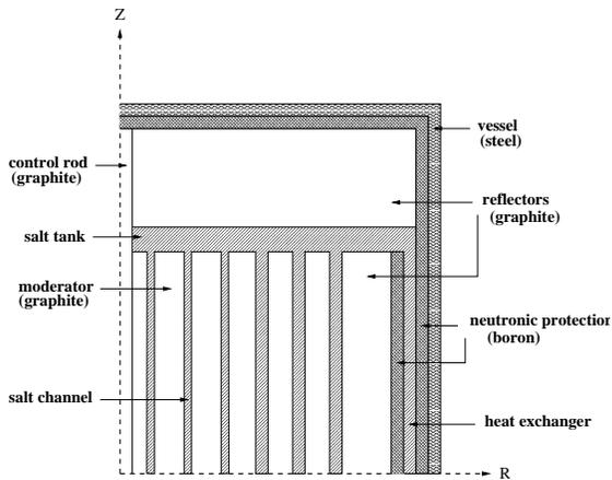
Figure 1: Schematic view of the simulated TMSR
