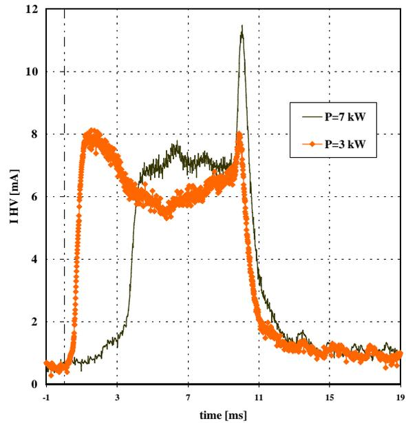
Fig. 5 : Example of the ECRIS HV current evolution with RF power in PHOENIX 28 GHz (Xe+O<sub>2</sub> mixing).
