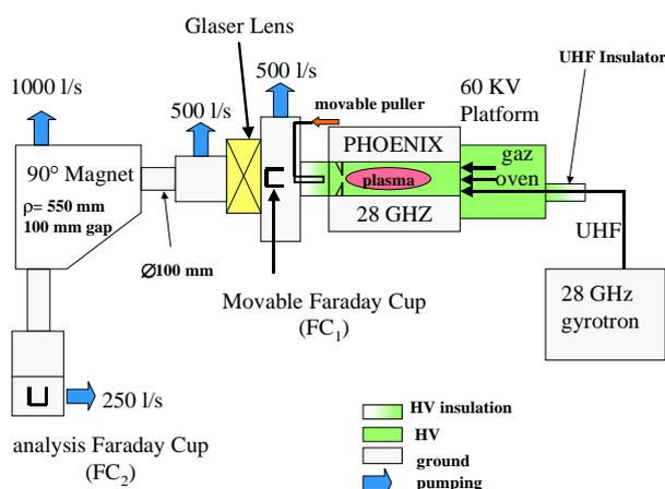
Fig 3 : Sketch of the high current PHOENIX bench.
