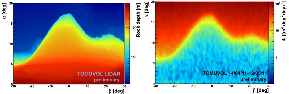
**Figure 2.** a) Material in front of the detector, evaluated from the LiDAR survey. b) The first flux measurements (here an example corresponding to 18.0 days of data taking with a  $1 \text{ m}^2$  detector) show the shadow cast in the atmospheric muon flux by the Puy de Dôme.
