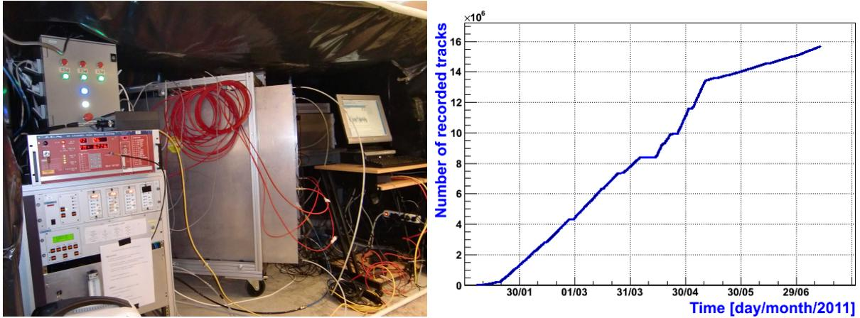
**Figure 1.** a) The detection setup at the Puy de Dôme. From left to right: (remote-)control station, HV supply and gas distribution system, GRPC detector and acquisition PC. b) Number of recorded muon tracks from January to July 2011 with three different detector configurations.
