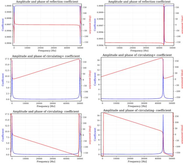
Figure 7. Variation of amplitude (blue) and phase (red) of reflection (top), forward-circulating (middle) and backward-circulating (bottom) coefficients for  $TEM_{00}$  (left) and  $TEM_{10}$  (right), in a model of VIRGO arm (finesse  $\sim 450$ ).
