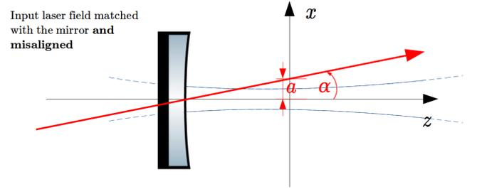
Figure 5. Misaligned beam on curved mirror.
