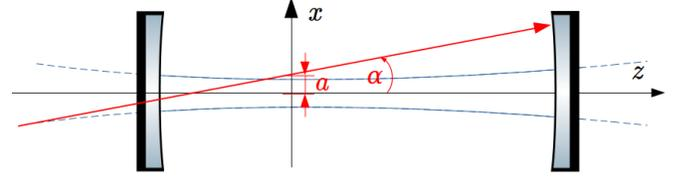
Figure 3. Misaligned beam.
