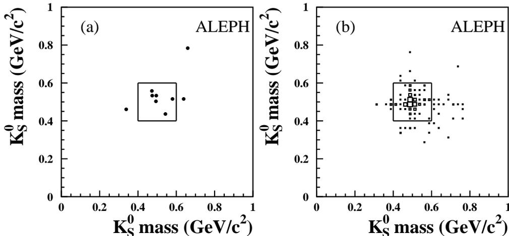
Figure 7: Scatter plots for the invariant  $K_S^0$  masses in the  $K_S^0 K_S^0 \pi^-$  mode: (a) data, (b) Monte Carlo predictions for signal are shown. The box indicates the  $K_S^0$  mass window for isolating the signal.
