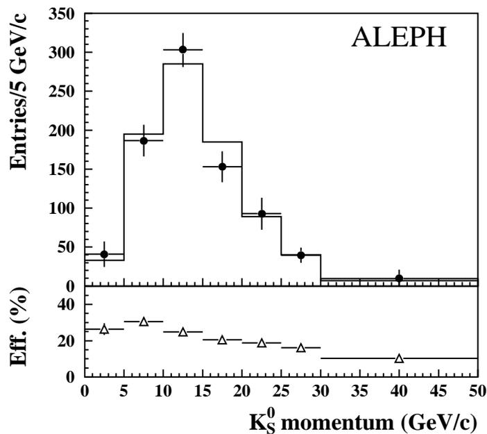
Figure 4: *Momentum distribution of the  $K_S^0$  candidates (points with error bars) in  $\tau$  decay. Monte Carlo prediction is given by the histogram. The  $K_S^0$  selection efficiency as a function of momentum is also shown below with triangles.*
