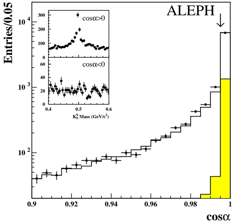
Figure 2:  $\cos\alpha$  distribution for data (black points). Monte Carlo predictions for all the neutral vertices and the true  $K_S^0$  signal are shown in the open and shaded histograms, which are normalized to the same luminosity as in data. The cut is indicated by the vertical arrow. The inset plots correspond to the neutral vertices with the correct (positive  $\cos\alpha$ ) and wrong (negative  $\cos\alpha$ ) solutions in the  $K_S^0$  finding algorithm.
