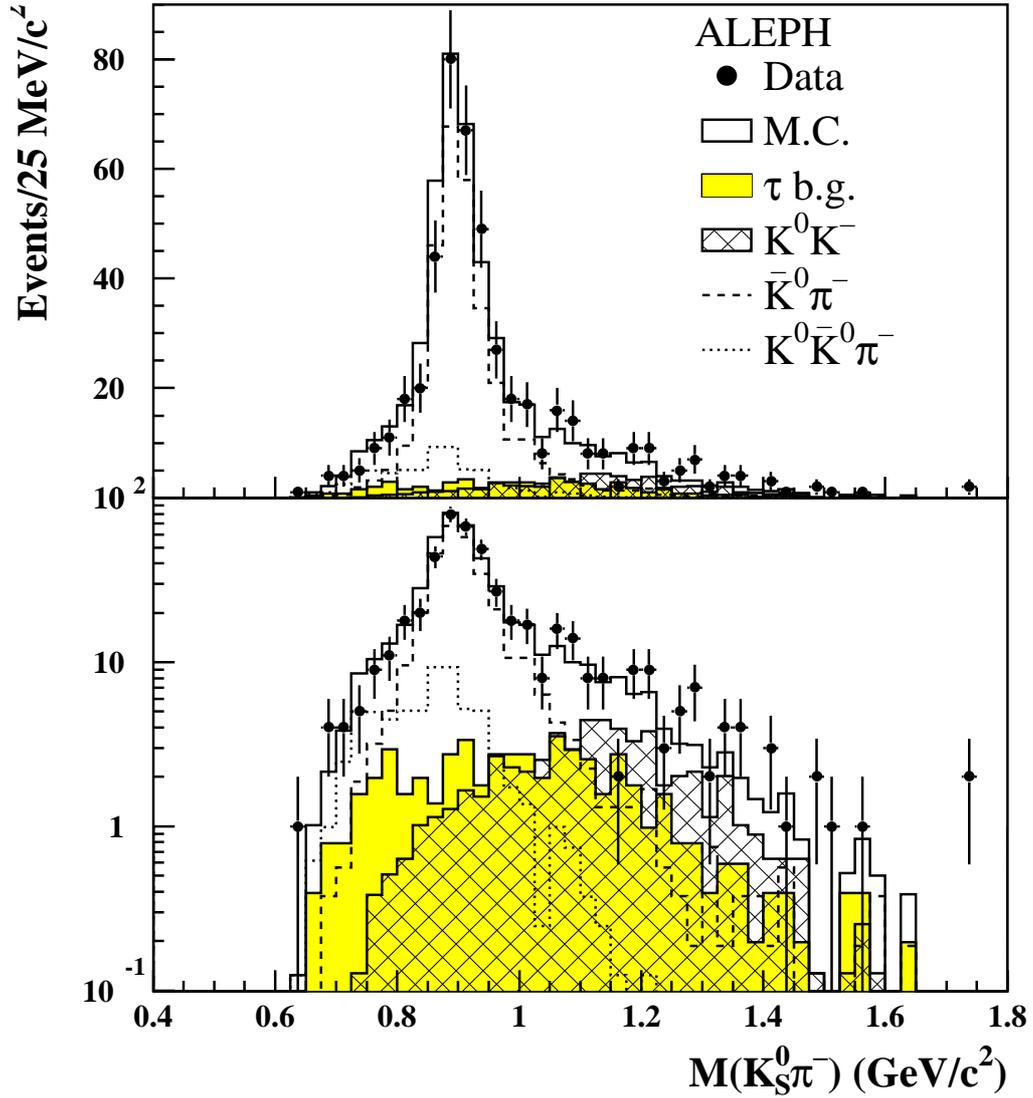
Figure 9: Invariant mass distribution of  $K_S^0 \pi^-$  candidates in the  $K_S^0 h^-$  sample for data (points with error bars) and Monte Carlo prediction (open histograms) [6, 7], respectively. The signal and  $\tau$  background contributions are also shown.
