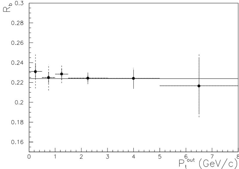
Figure 7:  $R_b$  versus the transverse momentum of the lepton. The bins are uncorrelated. The solid error bars indicate the statistical errors and the dashed ones the total errors. The horizontal line shows the result quoted in the text, obtained with the cut  $p_t^{\text{out}} > 1.5 \text{ GeV}/c$ .
