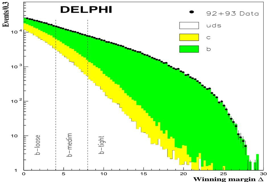
Figure 8: Distribution of the winning margin  $\Delta$  in the  $b$  tag categories for data and for simulation after correction. The different types of shading show the different flavour contributions to the simulated event sample. The simulation distributions are normalized to the data statistics. The values of the cuts defining the three  $b$  tag categories are also indicated.
