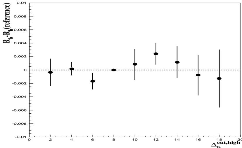
Figure 11: The value of  $R_b - R_b(\text{reference})$ , with its error, as a function of the cuts defining the three  $b$  categories.  $\Delta_b^{cut,low}$  was taken as half of  $\Delta_b^{cut,high}$ . The reference value of  $R_b$  is the value quoted in the text.
