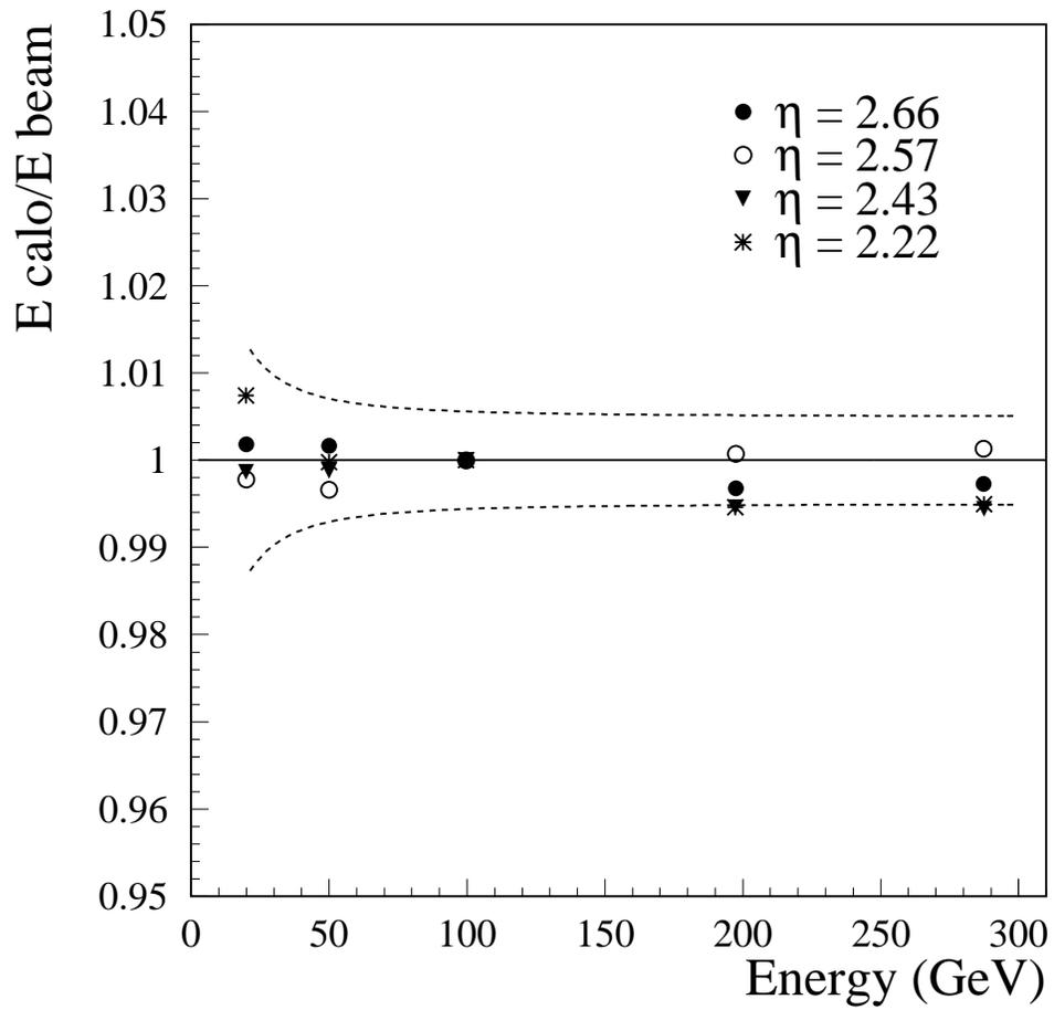
Figure 10: *Linearity of the calorimeter response for four cells at different  $\eta$  positions. The dashed lines represent the uncertainties in the nominal beam momentum.*
