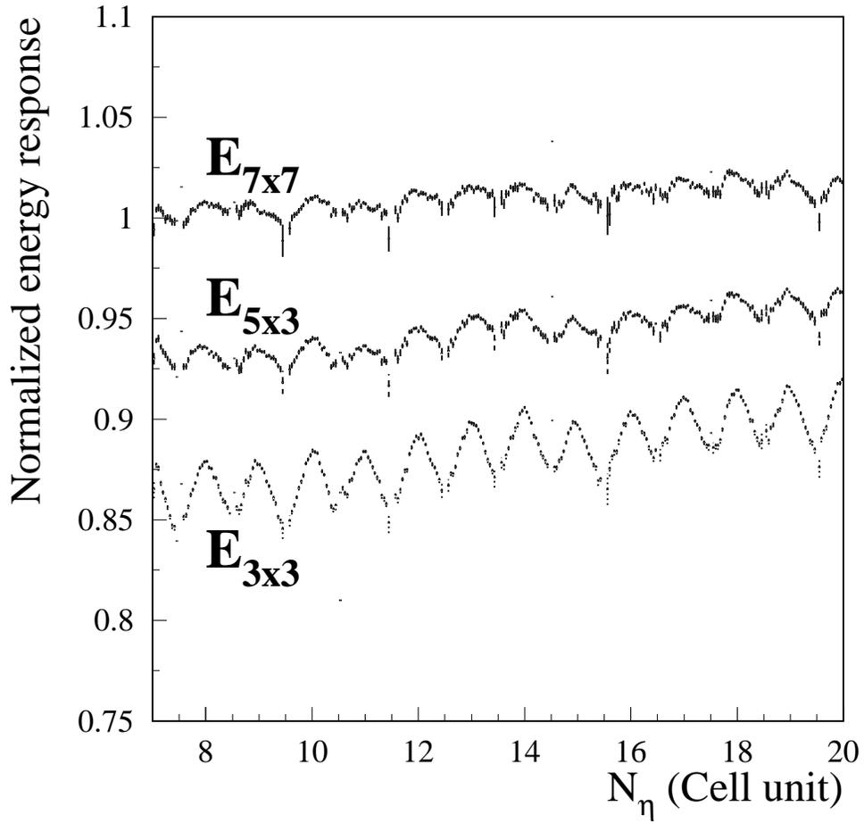
Figure 7: Reconstructed energy response, normalized to the energy in a cluster  $7 \times 7$  at  $N_\eta = 7$ , versus  $\eta$  for three different cluster sizes:  $(\eta \times \phi) = 3 \times 3, 5 \times 3, 7 \times 7$ .
