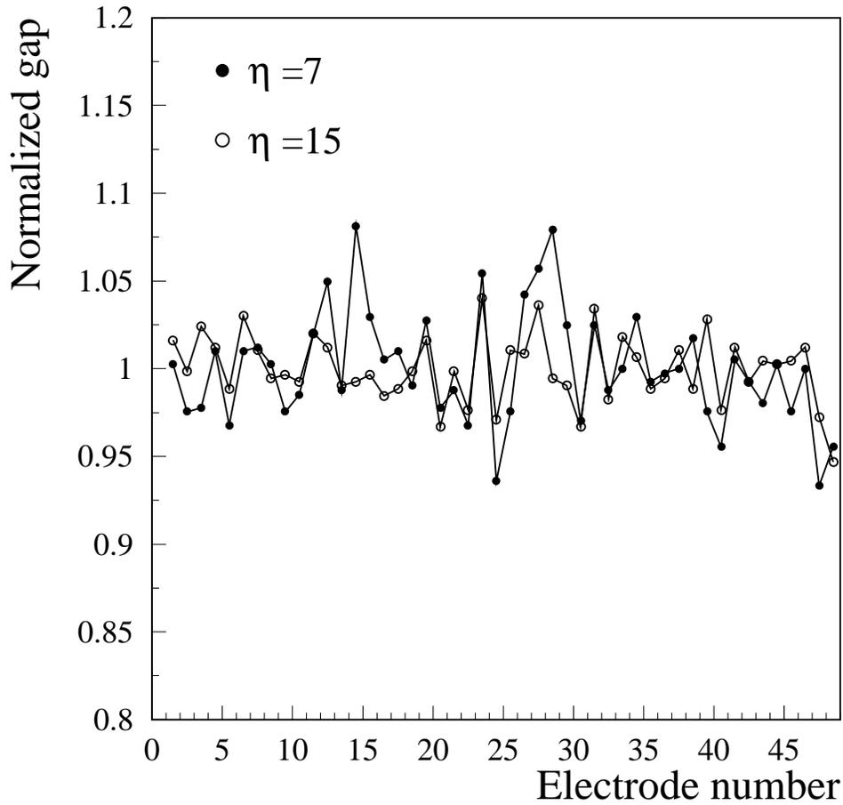
Figure 4: *Normalized capacitance as a function of the electrode number along two rows in  $\eta$ . The normalization is done with the mean value of each  $\eta$  row.*
