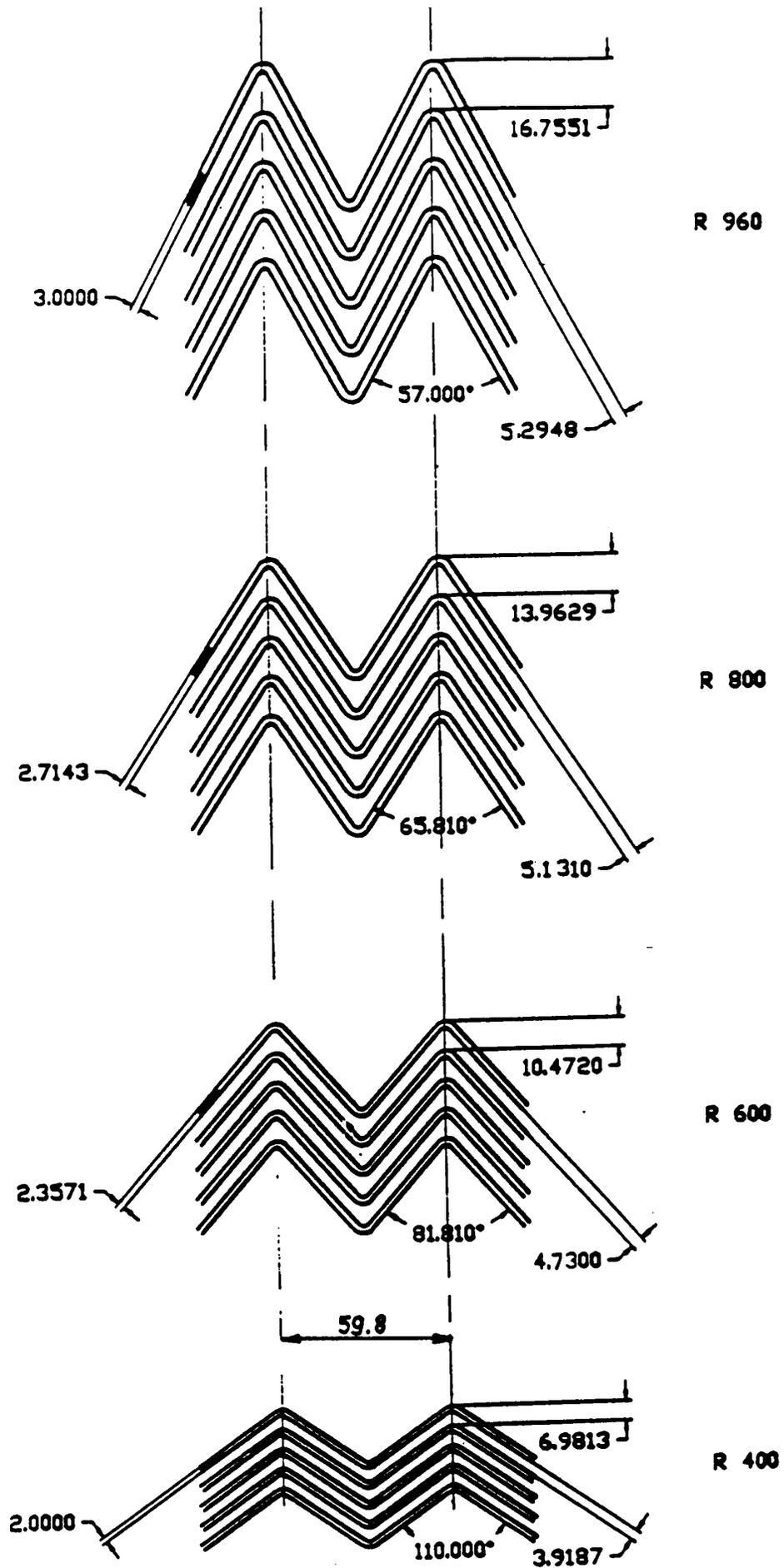
Figure 2: Converter plate profile at four values of the radius.
