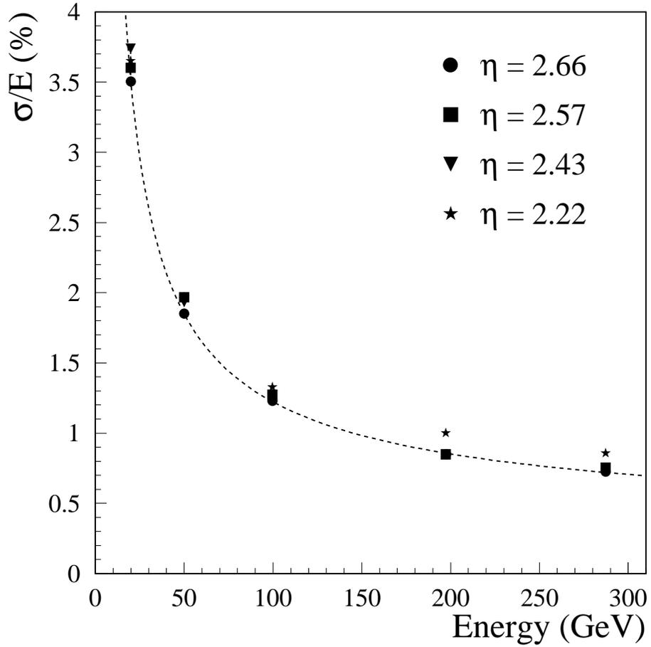
Figure 9: Energy resolution as a function of the incident beam energy at four different  $\eta$  values. The dashed line is the best fit to the data at  $\eta=2.66$ .
