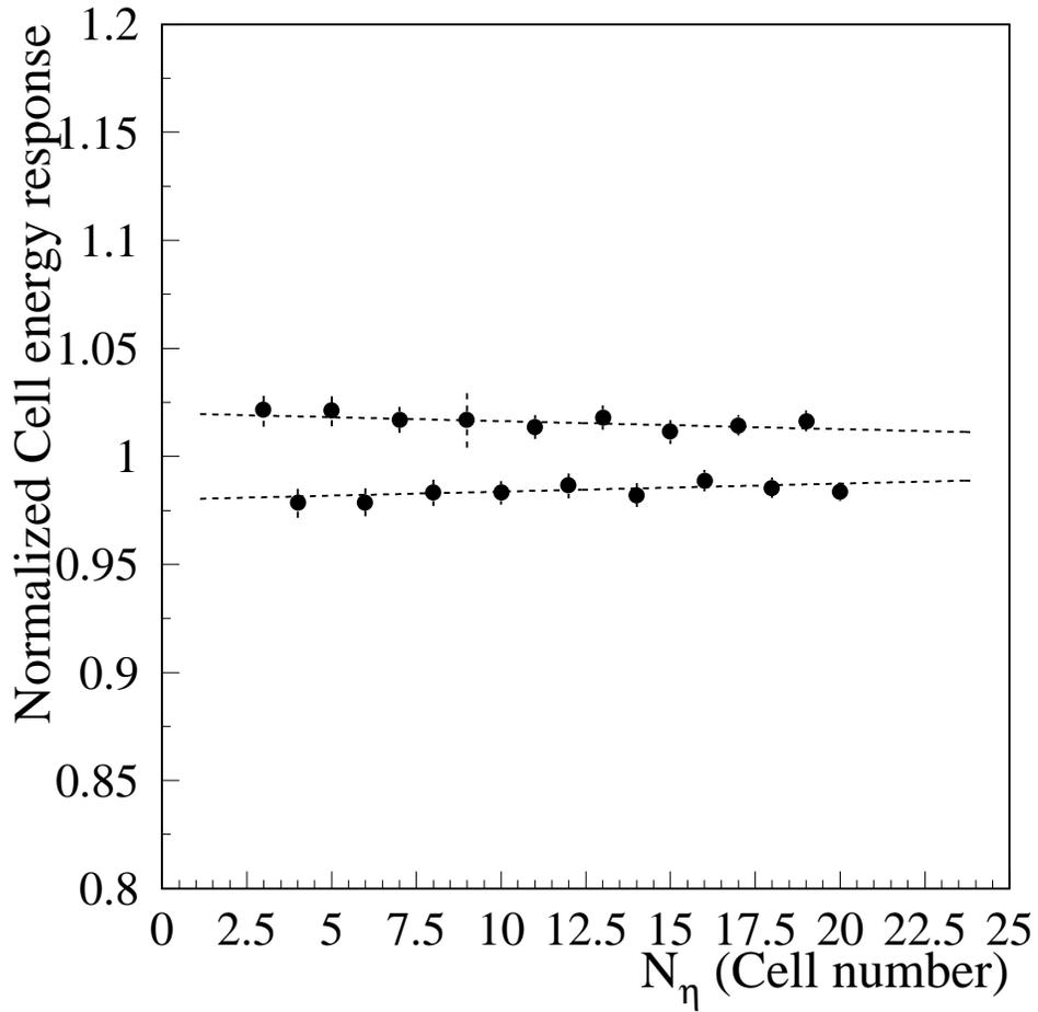
Figure 5: Normalized response of a cell as a function of the cell number in the  $\eta$  direction. The dotted lines correspond to linear fits to the odd and even cell response, used to correct an effect of the HV distribution.
