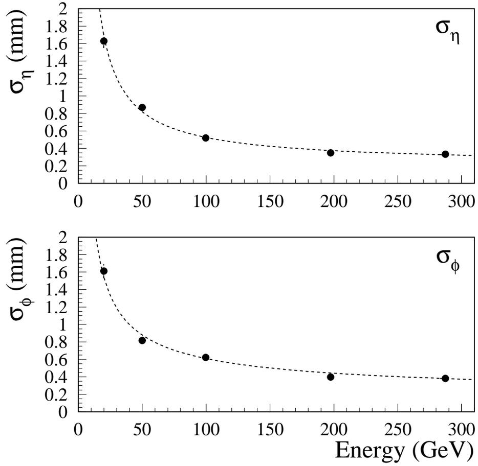
Figure 11: Position resolution in  $\eta$  direction at  $\eta=2.66$  (top) and position resolution in  $\phi$  direction at  $\eta=2.57$  (bottom) as a function of energy. The curves are the best fits to the data, according to eq. 4.
