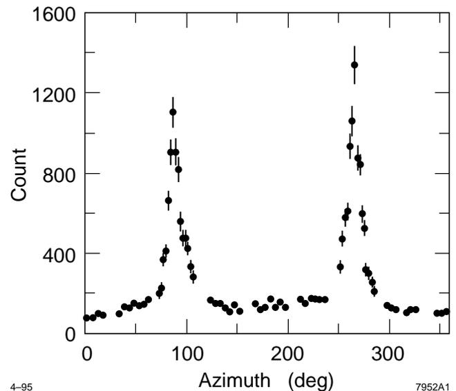
Figure 1. Angular distribution of  $\text{He}^+$  ions produced by beam ionization of Helium gas. The distribution is peaked in the horizontal direction ( $90^\circ$  and  $270^\circ$ ), indicating a flat beam.
