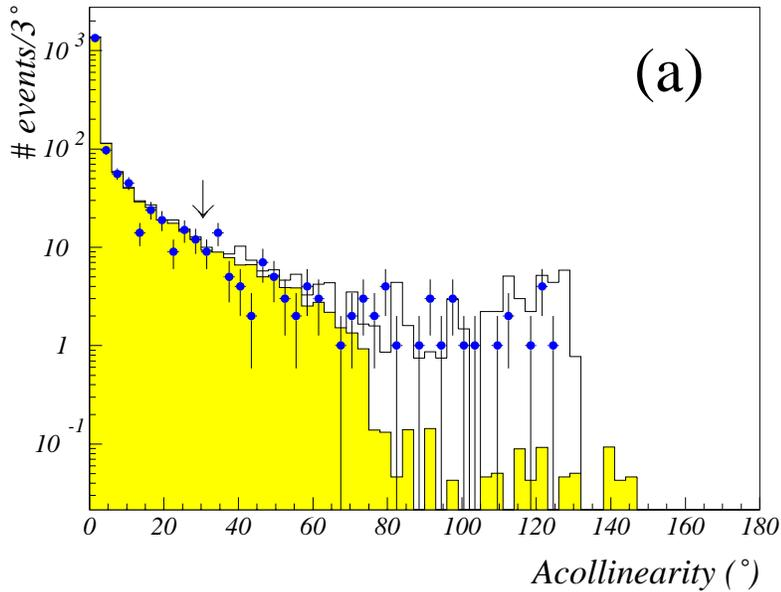
Figure 1: Acollinearity distribution for the  $\gamma\gamma(\gamma)$  sample selected at all centre-of-mass energies (dots), before imposing the  $30^\circ$  acollinearity cut (arrow). The histograms represent the QED  $e^+e^- \rightarrow \gamma\gamma(\gamma)$  simulation (grey area) and the remaining background (white area). The latter is mainly due to Compton ( $e^\pm\gamma$ ) events.
