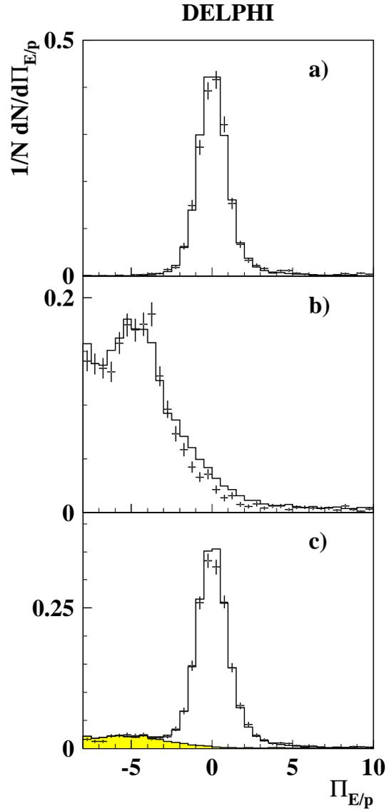
Figure 2: Distribution of the pull on  $E/p$  for the electron hypothesis,  $\Pi_{E/p}$ , for a) an electron test sample, b) a hadron test sample and c) after all other electron identification cuts. The points with error bars are real data, the unshaded histogram is simulated data, and the shaded histogram is the simulated background from  $\tau$  decays. The discrepancy in the HPC response to hadrons is clearly visible.
