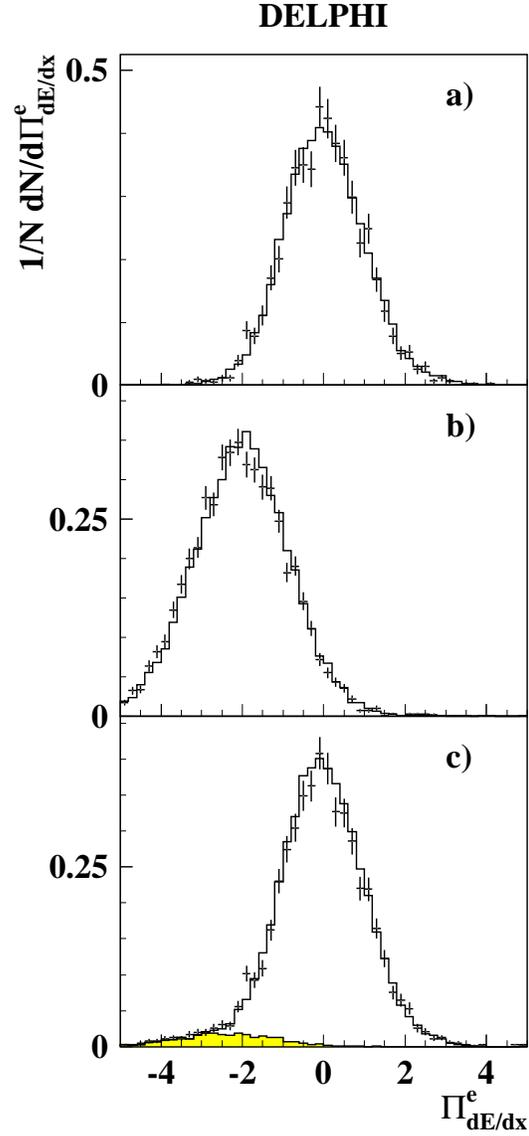
Figure 1: Distribution of the pull on  $dE/dx$  for the electron hypothesis,  $\Pi_{dE/dx}^e$ , for a) an electron test sample, b) a hadron test sample and c) after all other electron identification cuts. The points with error bars are real data, the unshaded histogram is simulated data, and the shaded histogram is the simulated background from  $\tau$  decays.
