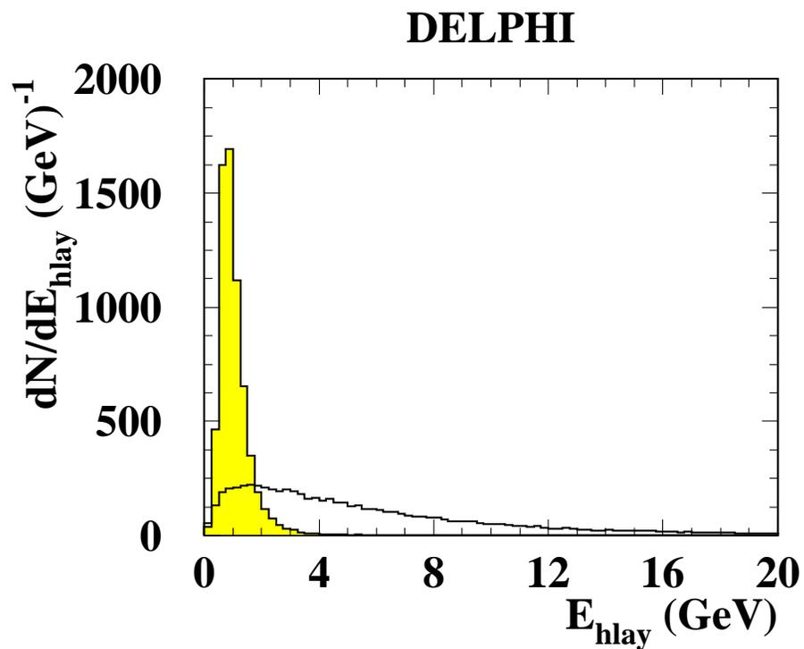
Figure 3: Distribution of the average energy per layer  $E_{hlay}$  in the hadron calorimeter for real data test samples of pions (unshaded histogram) and of muons (shaded histogram). Entries with  $E_{hlay} = 0$  have been suppressed.
