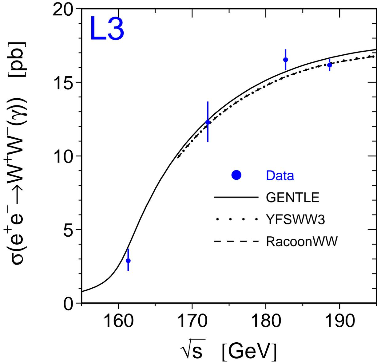
Figure 5: The CC03 cross section of the process  $e^+e^- \rightarrow W^+W^-(\gamma)$  as a function of the centre-of-mass energy. The published measurements at  $\sqrt{s} = 161, 172$  and  $183$  GeV, and the new measurement at  $\sqrt{s} = 189$  GeV are shown combining statistical and systematic uncertainties in quadrature. The curves show the SM expectation according to different calculations.
