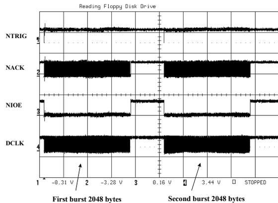
Figure 9: Read burst timing, 2 bursts of 2048 bytes.
