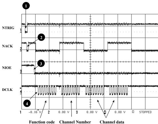
Figure 8: Read timing for a two bytes channel.
