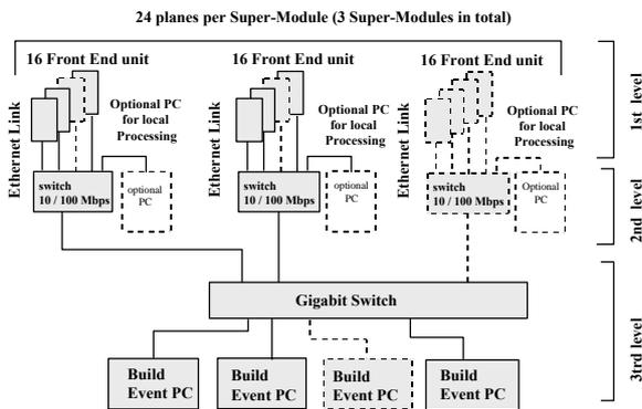
Figure 2: Network based Link acquisition system architecture.
