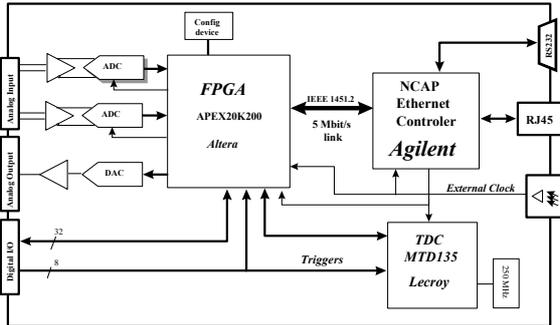
Figure 5: Ethernet Capable Front-end Module.
