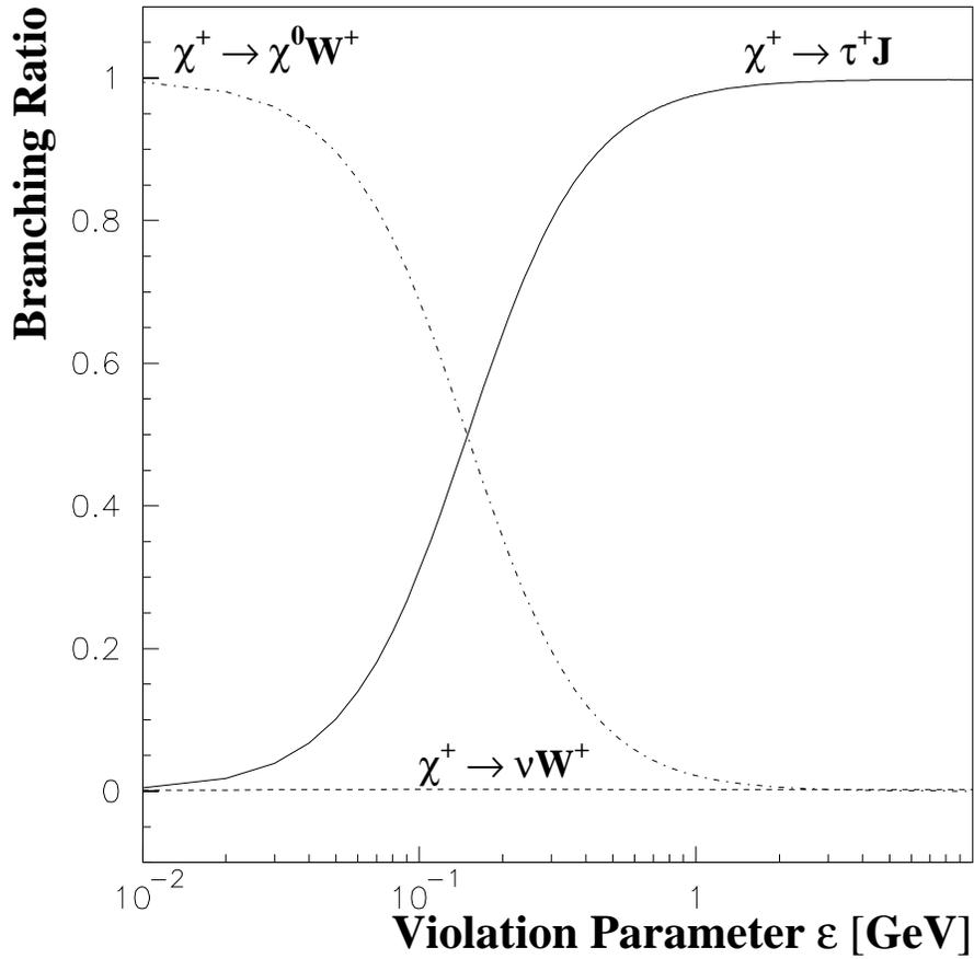
Figure 1: Chargino decay branching ratios as a function of the effective  $R$ -parity violation parameter  $\epsilon$  for  $\tan \beta = 2$ ,  $\mu = 100 \text{ GeV}/c^2$  and  $M_2 = 400 \text{ GeV}/c^2$ .
