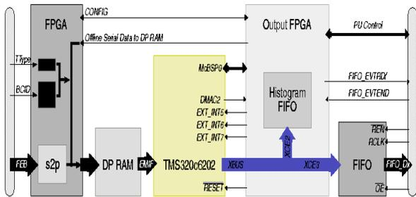
Figure 5 : Block diagram of PU 2.
