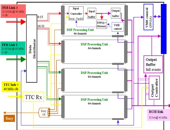
Figure 2 : The ROD demonstrator motherboard design.
