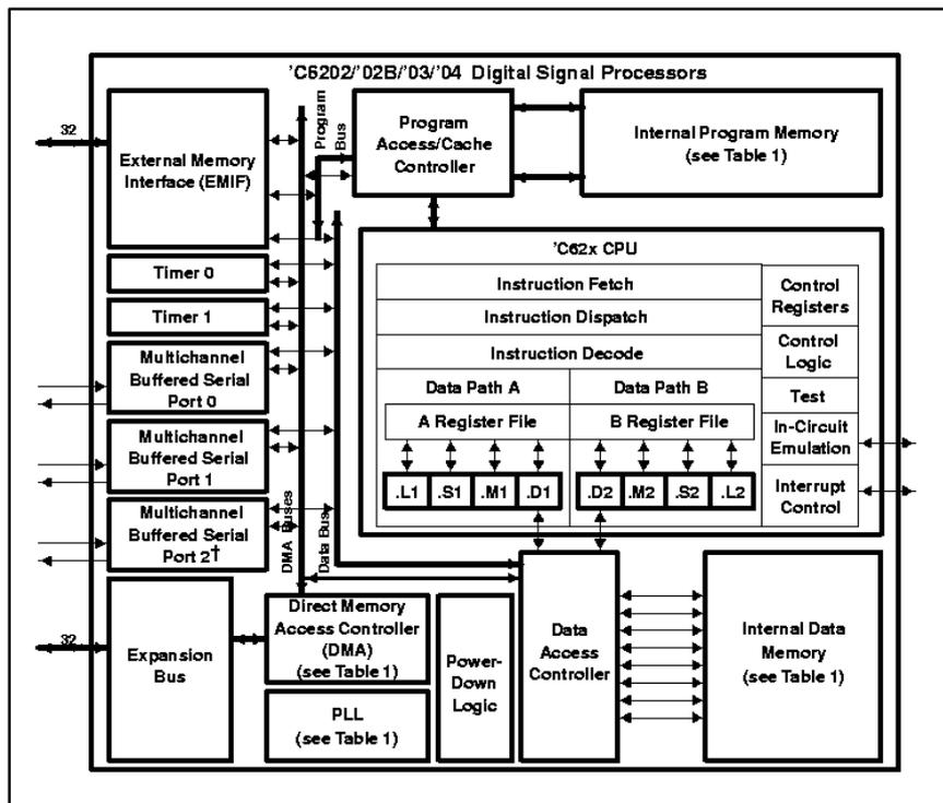
Figure 6 : The TMS 6202 DSP architecture
