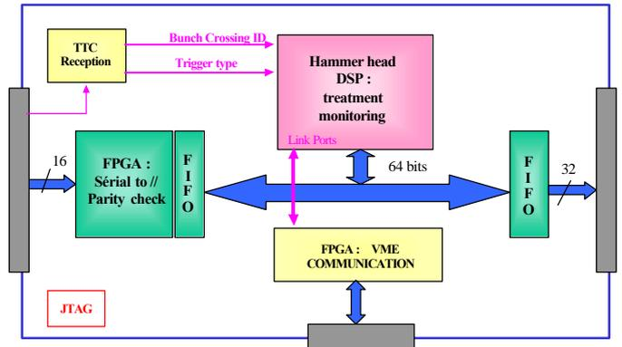
Figure 3 : The Analog Devices PU block diagram
