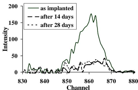
Figure 5: Evolution of the iodine concentration profiles at 300°C as function of the annealing time in autoclave.
