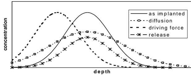
Figure 1: Effect of diffusion, driving force towards the surface and matter release on the profile evolution of implanted species
