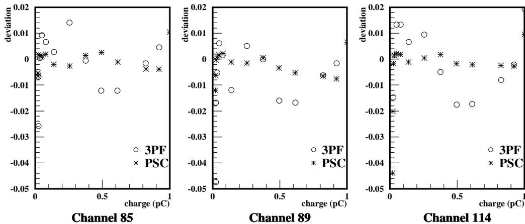
Figure 15: Deviation from linearity vs. amplitude for three different channels.
