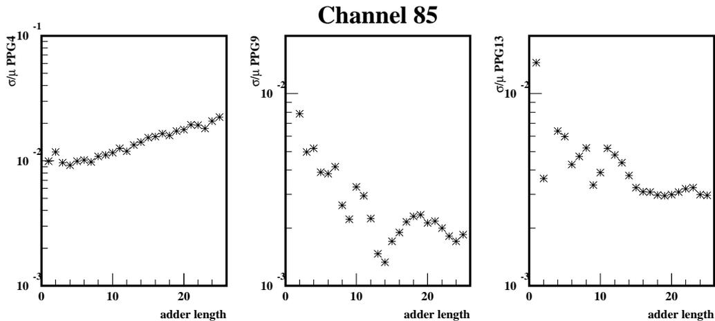
Figure 12: Resolution vs. adder length for three different PPG amplitudes, using pulse shape comparison lookup tables.
