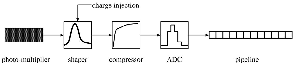
Figure 1: Block scheme of the read-out system. The digital pipeline has not been part of these tests.
