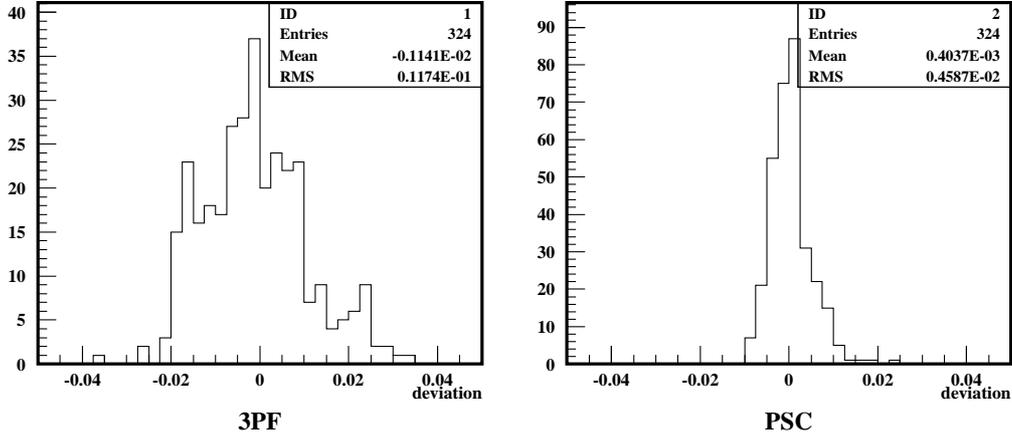
Figure 16: Deviations from linearity for all channels. PPG pulses with an amplitude below 0.025 pC are removed.
