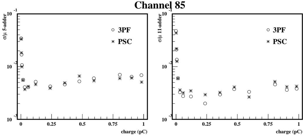
Figure 13: Resolution vs. PPG amplitude for adders of lengths 5 and 11.
