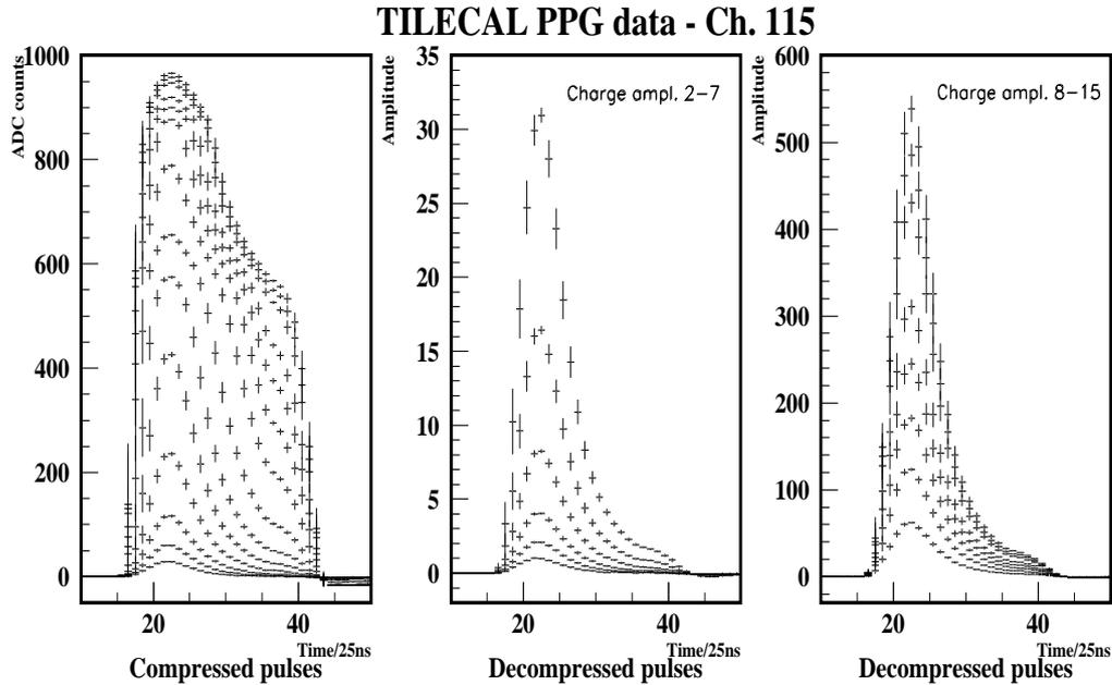
Figure 8: Average time frames for compressed (left) and decompressed (middle and right) PPG pulses.
