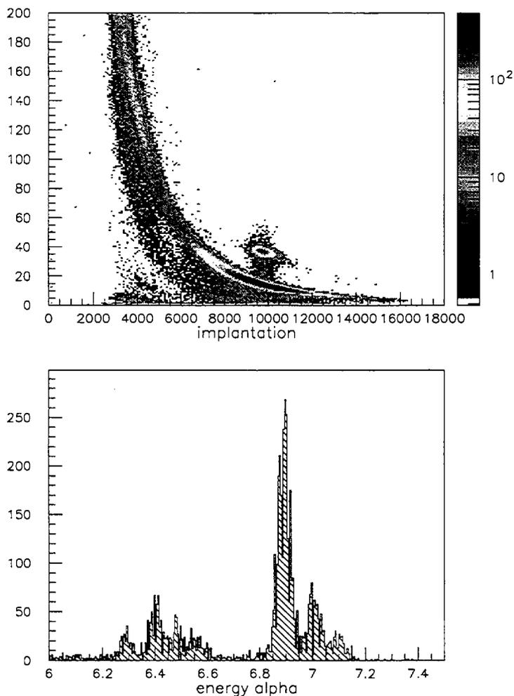
**FIGURE 2.** upper part: Energy versus Time-Of-flight spectrum for the system  $^{86}\text{Kr}$  (4.3 MeV/u) +  $^{121,123}\text{Sb}$ ; lower part:  $\alpha$  spectrum in anti-coincidence with the Time-Of-Flight.
