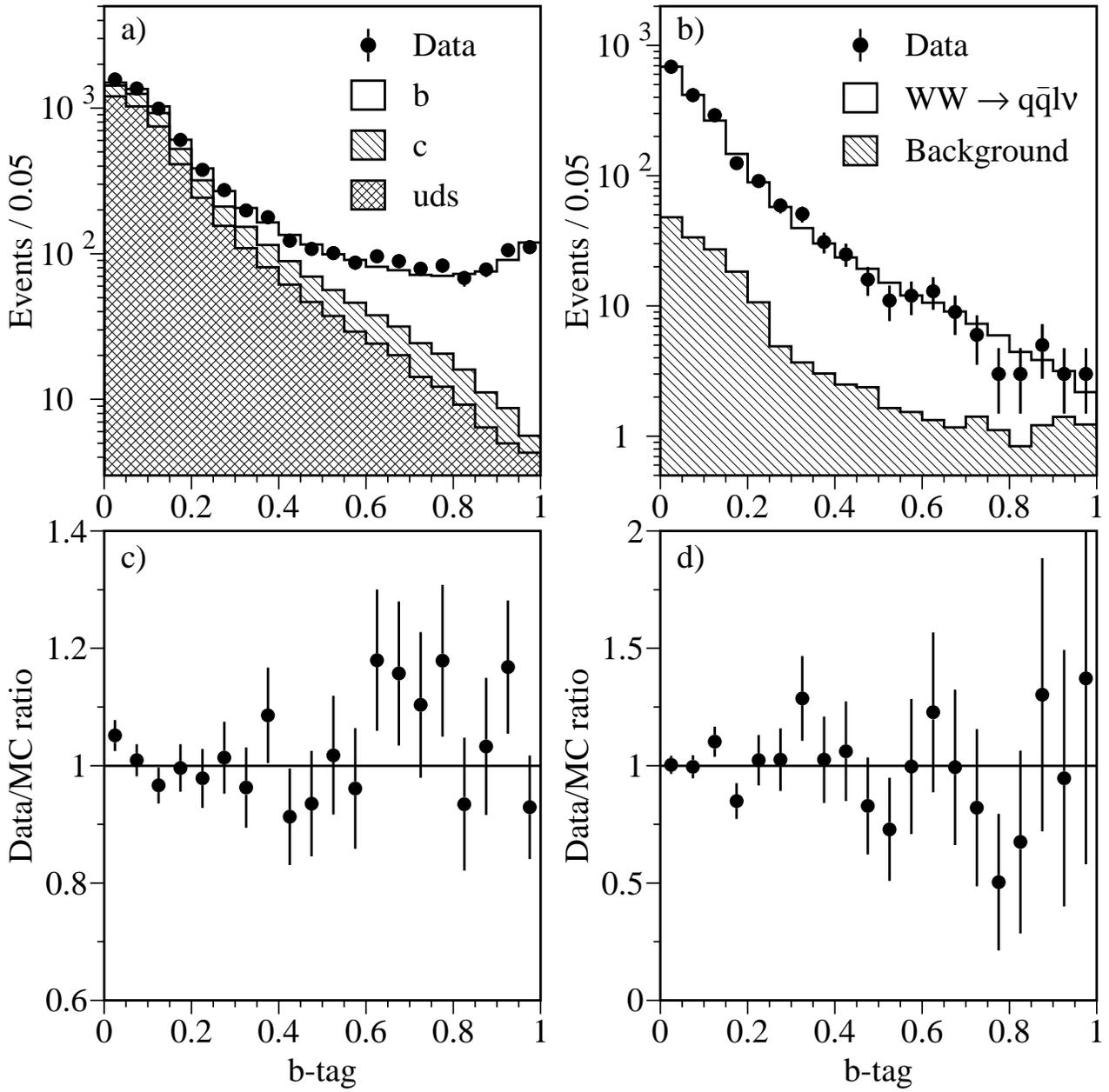
Figure 1: Distribution of the b-tag variable for jets in a sample of a)  $e^+e^- \rightarrow q\bar{q}(\gamma)$  and b)  $W^+W^- \rightarrow q\bar{q}l\nu$  events selected from the high-energy data collected in the year 2000. The data are compared to the simulation of Standard Model processes. The bin-by-bin ratio of the data to the simulated events is displayed in c) and d).
