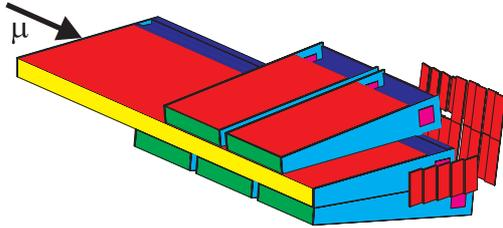
**Fig. 2.** The experimental setup. The muon beam indicated by the arrow enters in the center of 5.6 m long Module 0 from the left side. At the downstream end, the large calorimeter was surrounded below by three 1-meter long small calorimeters and above by two of them
