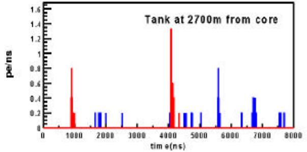
**Figure 1-a.** Distribution of photoelectrons for one PMT as a function of time for a 500 EeV vertical proton shower detected in tanks at 500, 1000 and 2500 m from the shower core. The blue line corresponds to the total distribution and the red filled spectrum shows the muon contribution.
