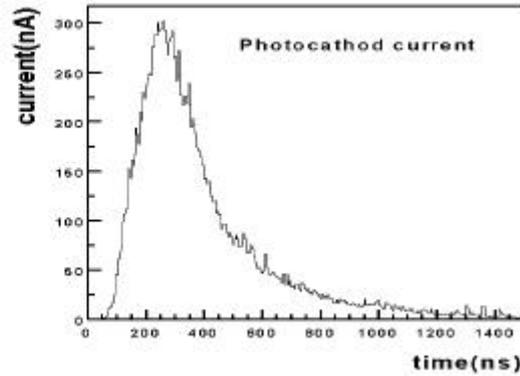
**Figure 4-b** Photocathode current for the same PMT
