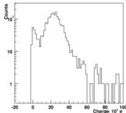
**Figure 3.** Charge spectrum measured from telescope triggered muons. Absorbing material was put between the scintillators to eliminate the soft electromagnetic background. An oscilloscope with a sampling of 1GHz was used for the data acquisition. In this setup, one VEM corresponds to  $2.3 \cdot 10^7 e$ .
