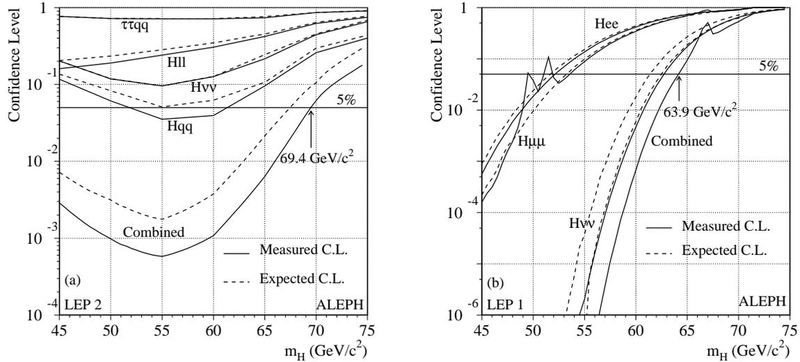
Figure 8: The measured (full curves) and expected (dashed curves) confidence levels for each of the final states, and their combination, (a) at high energy and (b) at LEP 1. The  $H\tau^+\tau^-$  and  $\tau^+\tau^-q\bar{q}$  analyses are combined into a single  $\tau^+\tau^-q\bar{q}$  result.
