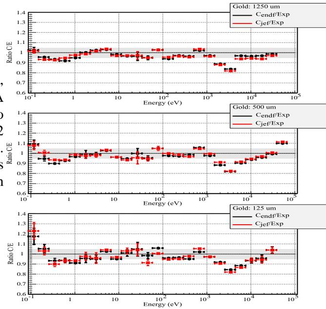
Figure 9: ENDF/BVI and JEF2.2 simulation to experiment ratio for 1250  $\mu\text{m}$ , 500  $\mu\text{m}$  and 125  $\mu\text{m}$  Gold samples in the energy range from 0.1 eV to 40 keV. The large grey box around  $C/E = 1$  corresponds to an uncertainty of 5%.
