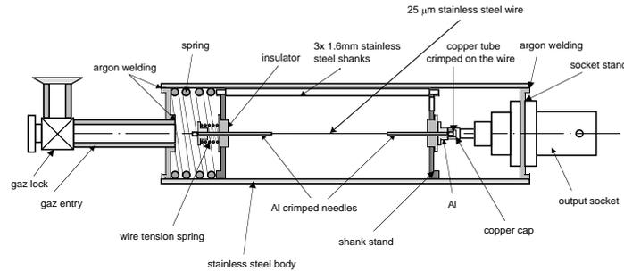
Figure 3: Mechanical structure of the  $^3\text{He}$  gas proportional counter detector
