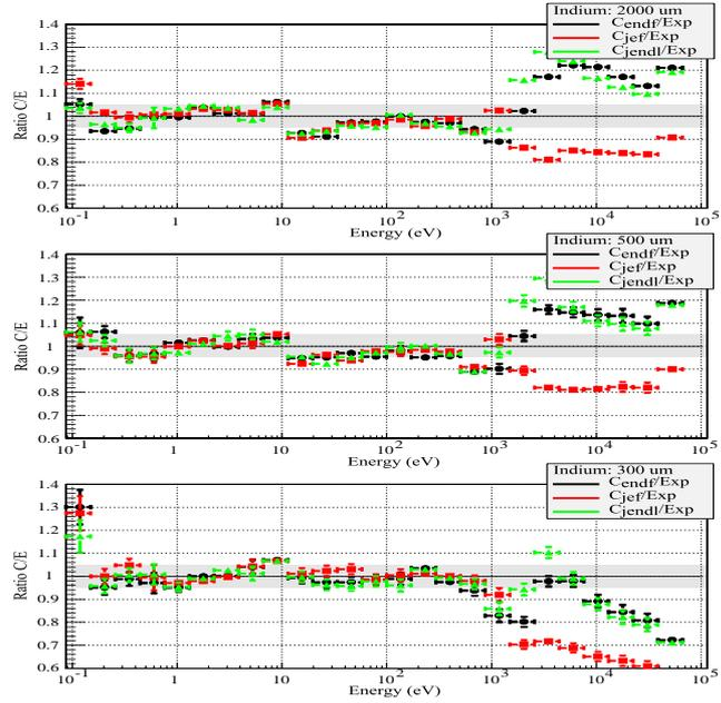
Figure 11: ENDF/BVI, JEF2.2 and JENDL3.2 simulation to experiment ratio for 2000  $\mu\text{m}$ , 500  $\mu\text{m}$  and 300  $\mu\text{m}$  Indium samples in the energy range from 0.1 eV to 40 keV
