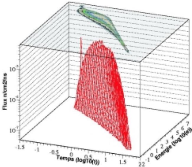
$$\bar{E} = \frac{K}{(t + t_0)^2} \quad \begin{matrix} K = 166 \pm 1 \text{ keV} \mu\text{s}^2 \\ t_0 = 0.5 \mu\text{s} \end{matrix}$$
