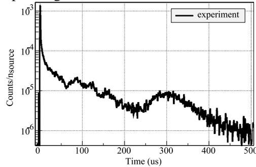
Figure 5: Timing spectra of the  $^{233}\text{U}$  detector:  $200 \mu\text{g}/\text{cm}^2$
