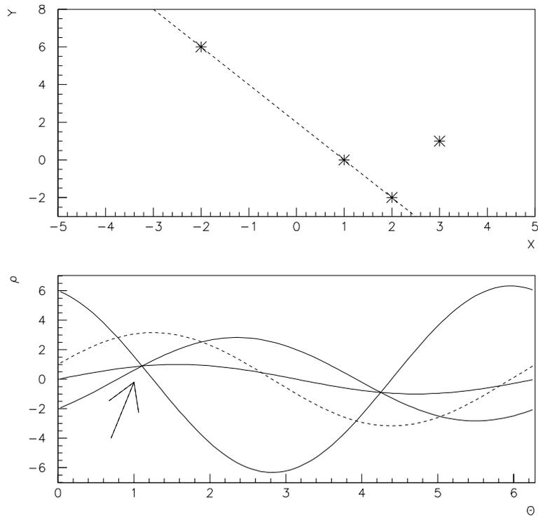
Figure 1: Illustration of the Hough Transform method with a) four points three of them on the line defined by  $y = -2x + 2$  and one outside b) the associated curves of the four points in the  $(\theta, \rho)$  plane.
