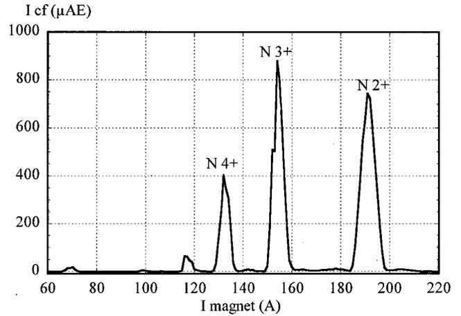
FIG. 3. N<sup>3+</sup> up to 900 μA with  $\varnothing$  2 mm extraction hole at 48 kV.
