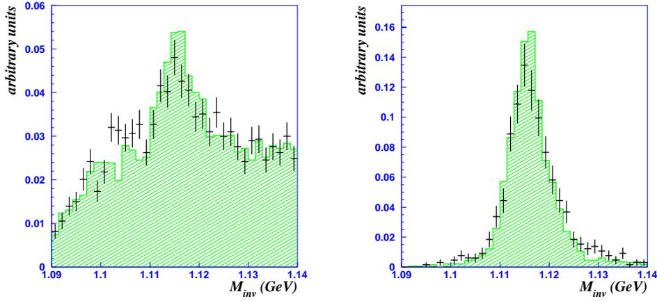
Fig. 2. Normalized invariant mass distributions in both data (points with error bars) and MC (histogram) calculated for  $V^0$  vertices under the assumption of a  $\bar{\Lambda}$  decay before (left) and after (right) the  $V^0$  identification procedure.
