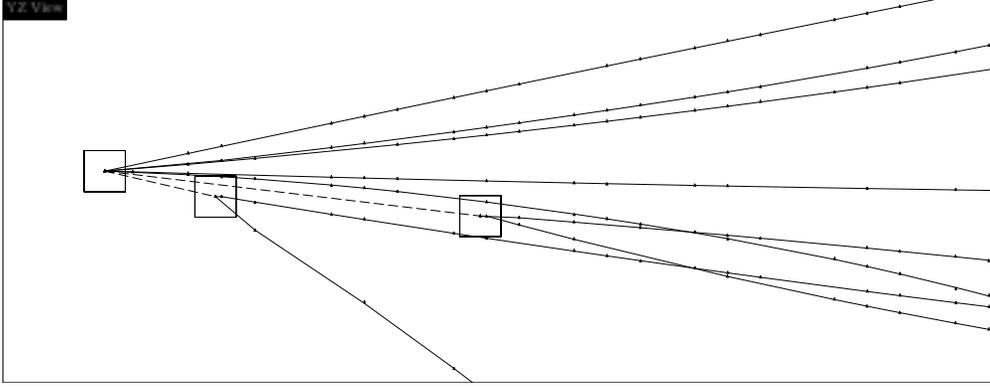
Fig. 1. A reconstructed data event containing 2  $V^0$  vertices identified as  $\Lambda$  and  $\bar{\Lambda}$  decays by our identification procedure. The scale on this plot is given by the size of the vertex boxes ( $3 \times 3 \text{ cm}^2$ ).
