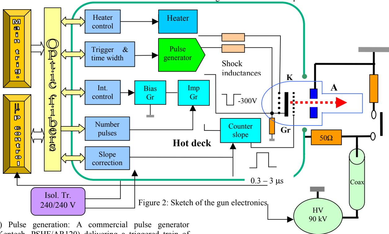
Figure 2: Sketch of the gun electronics
