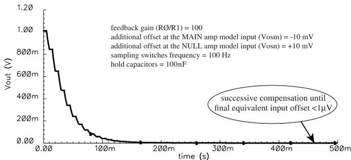
Figure 5: offset compensation step by step
