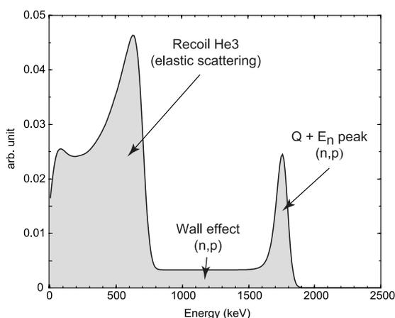
Figure 7. Typical response spectrum of <sup>3</sup>He proportional counter to 1 MeV monoenergetic neutrons.
