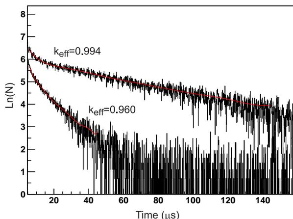
Figure 3. Logarithmic time spectra obtained with a U5 fission chamber in the fuel zone of MASURCA for two subcriticality levels  $k_{eff} = 0.994$  and  $k_{eff} = 0.960$ . Plain curves are polynomial fits of the spectra.
