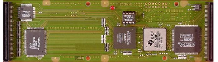
Figure 3: PU with Texas Instruments DSP C6203.
