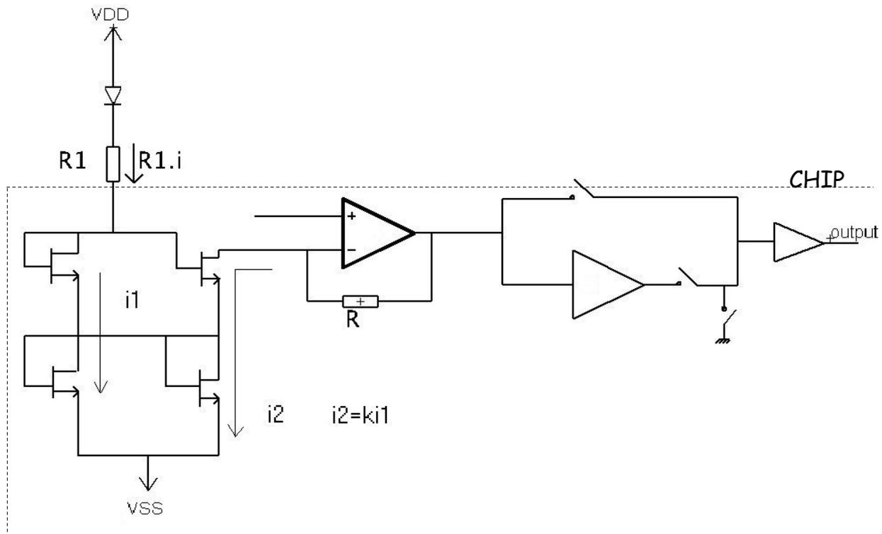
Figure 3. Pedestal Level Input Schematic
