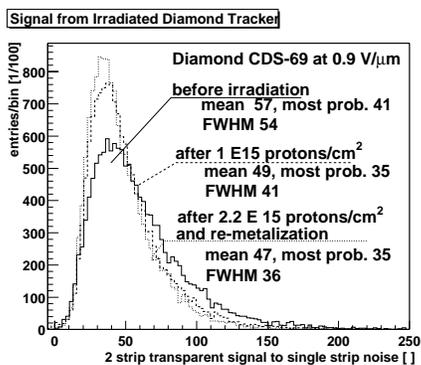
Fig. 4. Transparent 2-strip charge signal-to-noise distributions before (solid line), after proton irradiations with  $1 \times 10^{15} \text{ p/cm}^2$  (dashed line) and after  $2.2 \times 10^{15} \text{ p/cm}^2$  (dotted line).
