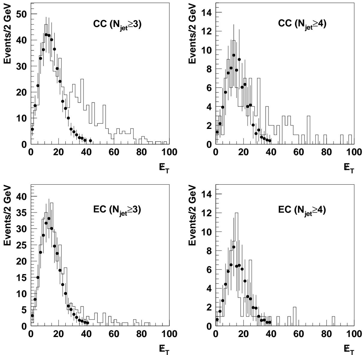
FIG. 4.  $\cancel{E}_T$  spectra of sample 2 (points) normalized to sample 1 (histograms) in the region of  $0 \leq \cancel{E}_T \leq 14$  GeV. The normalizations are done for the fake electron in the CC and EC, respectively. The errors are statistical only.
