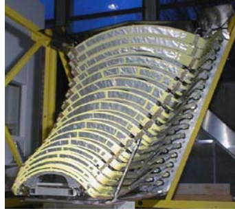
Figure 9. One octant with the 16 arc-shaped scintillators and light guides installed in the mechanical support.
