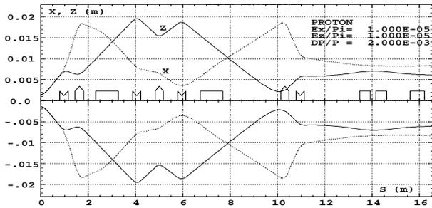
Figure 3: Beam envelopes in the MEBL (proton case).
