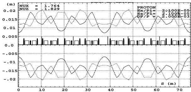
Figure 4: 7 MeV p-beam stored envelopes after injection.
