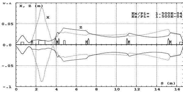
Figure 2: Beam envelopes in the LEBL (no space charge).
