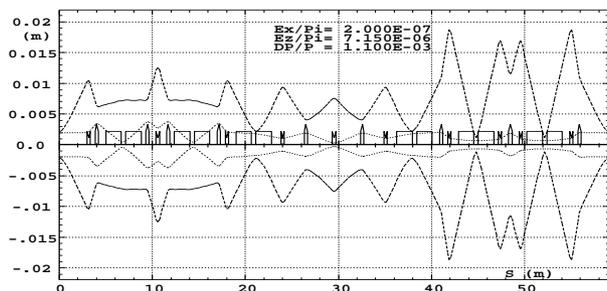
Figure 7: Typical envelopes in the 59 m long vertical beam line.
