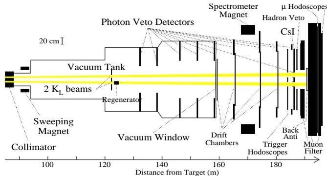
FIG. 1: The KTeV detector configured for measuring  $\text{Re}(\epsilon'/\epsilon)$ .
