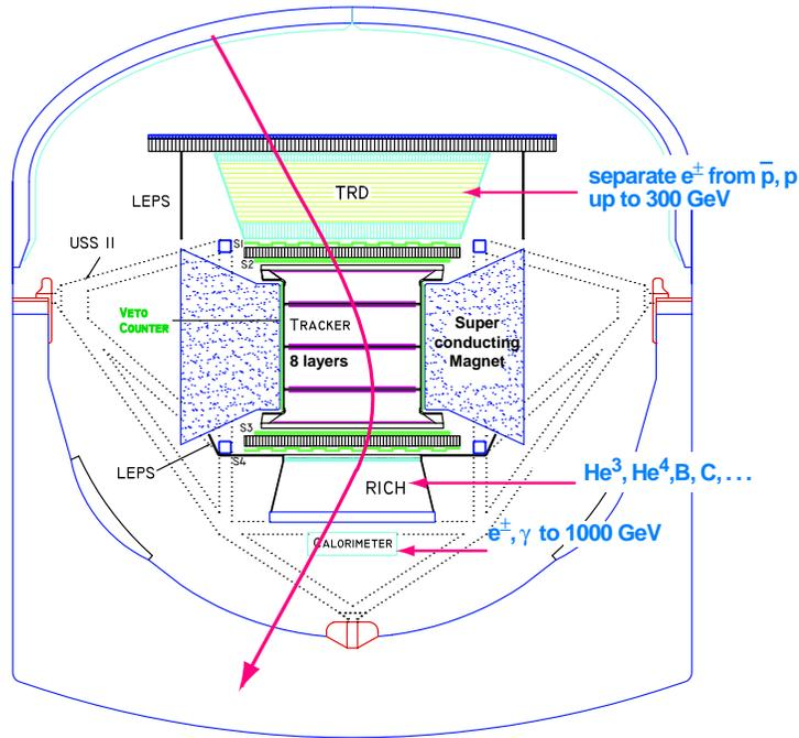
Figure 1. Schematic of AMS-02 detector.
