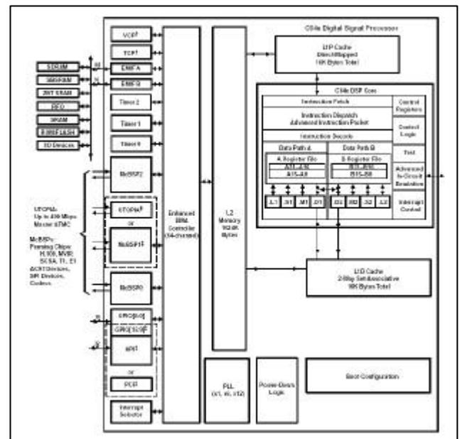
Figure 4 : The TMS320C6414 architecture
