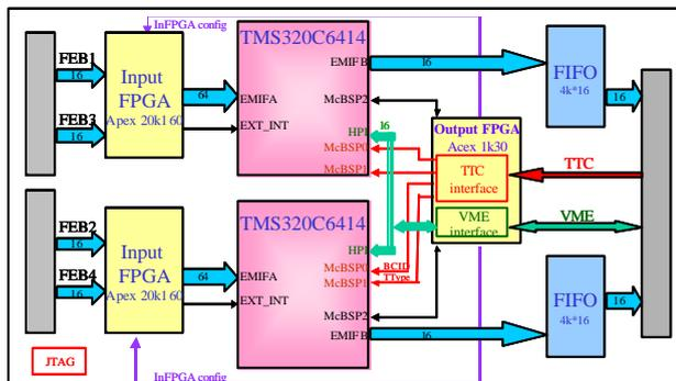
Figure 3 : The Processing Unit block diagram
