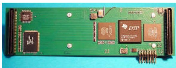
Figure 6 : The single DSP PU prototype.
