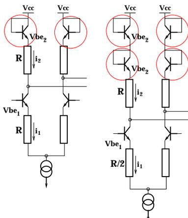
Figure 3: serial compensation
