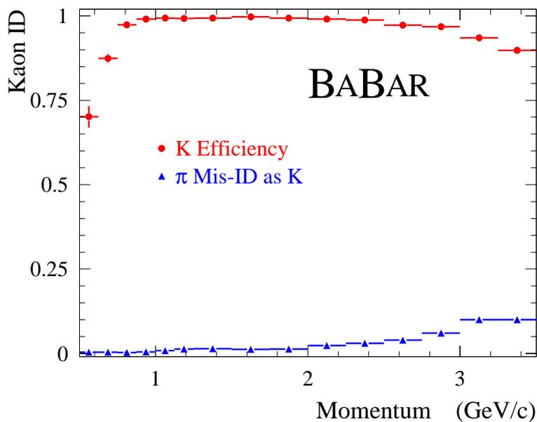
Figure 11: Efficiency and misidentification probability for the selection of charged kaons as a function of track momentum, for a particular choice of particle selection criteria. The data use  $D^0 \rightarrow K^- \pi^+$  decays selected kinematically from inclusive  $D^*$  production.
