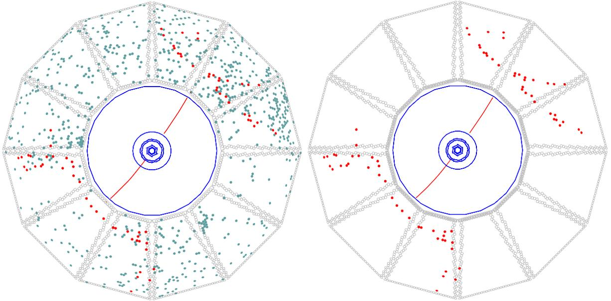
Figure 3: Display of an  $e^+e^- \rightarrow \mu^+\mu^-$  event reconstructed in *BABAR* with two different time cuts. On the left, all DIRC PMTs with signals within the  $\pm 300$  ns trigger window are shown. On the right, only those PMTs with signals within 8 ns of the expected Cherenkov photon arrival time are displayed.
