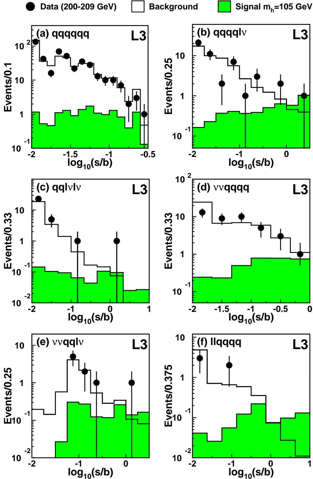
Figure 3: Distributions of the final variable for data, background Monte Carlo and signal Monte Carlo at  $m_h = 105$  GeV. All centre-of-mass energies and subchannels are combined. The final variable is displayed in bins of  $\log_{10}(\frac{\text{signal}}{\text{background}})$ .
