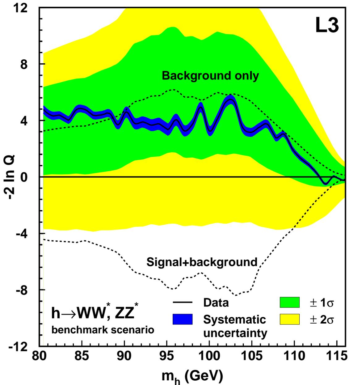
Figure 4: Log-likelihood ratio plot for the combined  $h \rightarrow WW^*, ZZ^*$  search. The dashed lines represent the value of the expected background-only and signal+background distributions. The shaded regions around the background-only line indicate the  $\pm 1\sigma$  and  $\pm 2\sigma$  regions. The solid line indicates the observed values. The bands around the observed sensitivity represent the effects of systematic uncertainties.
