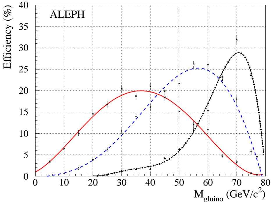
Figure 11: The three parametrized selection efficiencies for  $m_{\tilde{t}} = 80 \text{ GeV}/c^2$  (full curve, large  $\Delta M$  selection; dashed curve, intermediate  $\Delta M$  selection; and dot-dashed curve, small  $\Delta M$  selection) as a function of  $m_{\tilde{g}}$ . The dots with error bars show the actual efficiencies obtained from the individual simulated samples.
