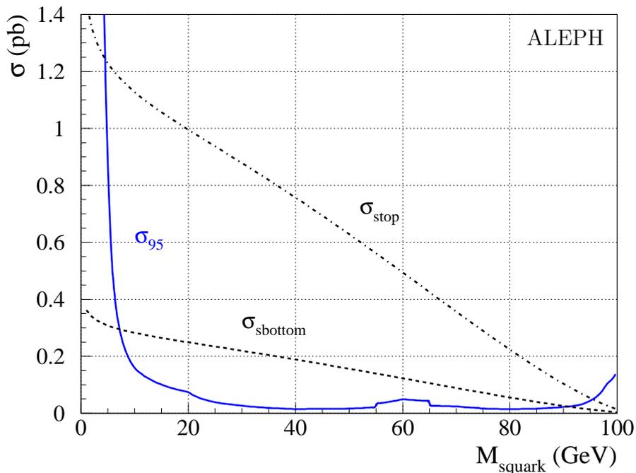
Figure 9: The production cross sections for  $e^+e^- \rightarrow \tilde{t}\tilde{t}^*$  and  $\tilde{b}\tilde{b}^*$  at  $\sqrt{s} = 209$  GeV, as a function of the squark mass. Also shown is the observed 95% C.L. upper limit on the cross section, derived from the stable stop search of Ref. [3].
