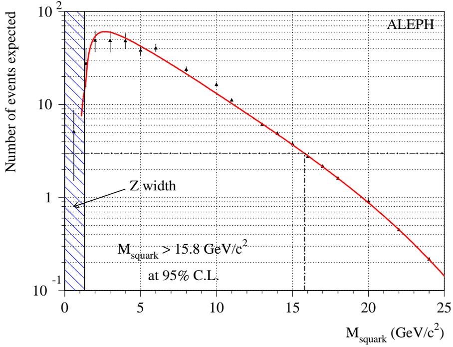
Figure 7: The number of  $q\bar{q}q\bar{q}$  events expected to be selected in the LEP1 data as a function of the squark mass (full curve). The triangles with error bars show the individual values obtained from each of the simulated signal samples. Also shown is the region excluded by the Z lineshape measurement (hatched region), and the lower limit on the squark-LSP mass (dot-dashed lines).
