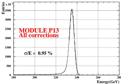
Fig. 3. Energy resolution for a whole barrel module
