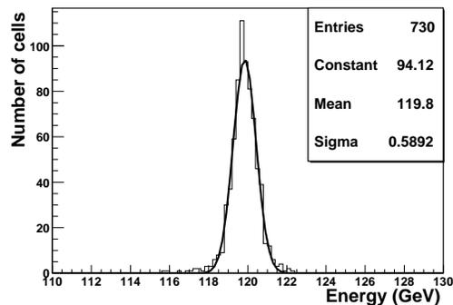
Fig. 2. Response uniformity of an end-cap module
