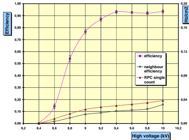
Fig. 4. RPC efficiency for the gas mixture Ar 49% Isob 7% Forane 40% SF<sub>6</sub> 4%
