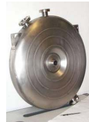
Fig. 5 Superconducting re-entrant structure (INFN-Legnaro)
