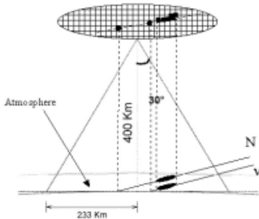
**Fig. 1.** Neutrino shower and hadronic shower as imaged by the EUSO focal surface detector. Note as the Čerenkov signature permits to resolve high penetrating neutrino from quick interacting primary hadron.
