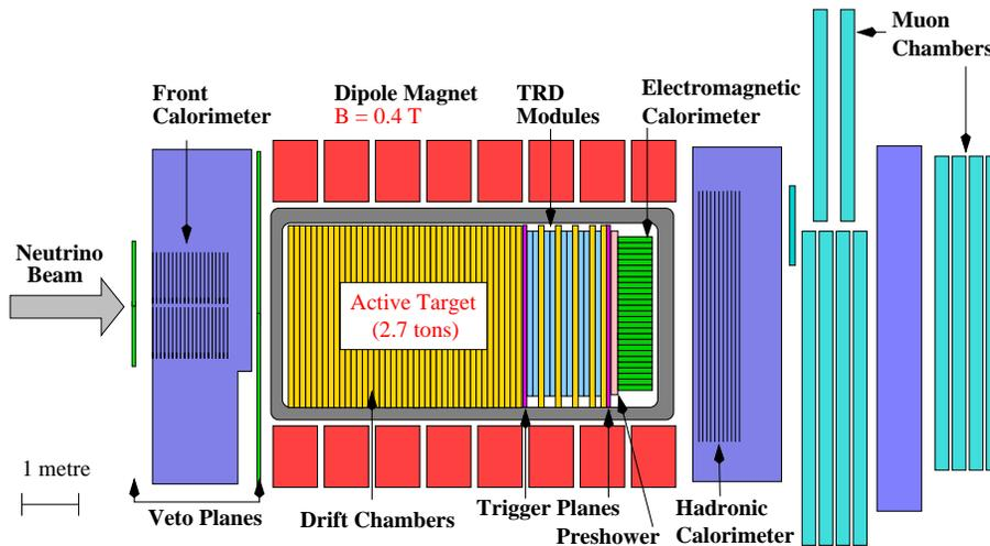
Fig. 1. Side view of the NOMAD detector.
